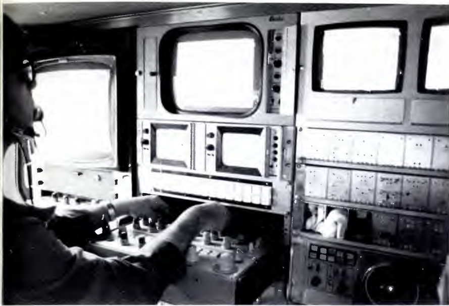
Control and monitoring equipment fills forward wall of truck cabin in back of driver. Operator sits with back near studio doors.
