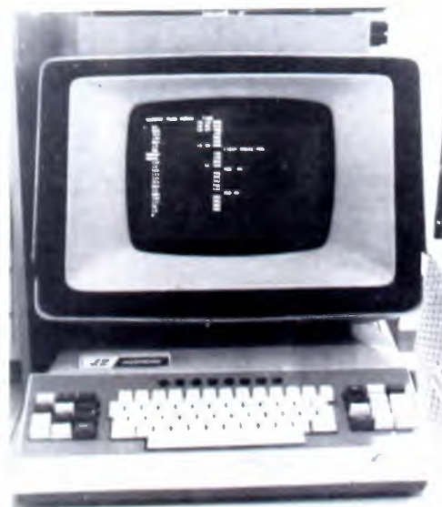
Close up of the Vital Vimax-27 console. The 27 events that this system handles are more than adequate for WLWD's chief engineer, Harold Thompson.
