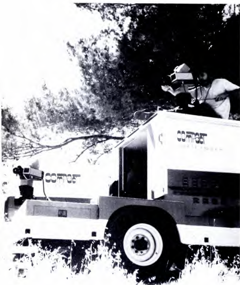
Camera-studio truck operating with camera on roof, another on open rear platform. Complete control studio is inside roofed part of truck. Power truck can be seen in background.
